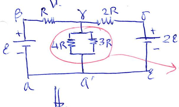
$$R_{100\Omega} = \frac{1}{\frac{1}{4R} + \frac{1}{3R}} \Rightarrow R_{100\Omega} = 1.71R$$
