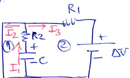
βεδόνος 1:  $\Delta V_c - I_1 R_2 = \phi \Rightarrow \Delta V_c = I_1 R_2$
