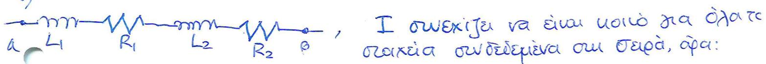
$$-L \frac{dI}{dt} - IR_1 - L_2 \frac{dI}{dt} - IR_2 = - (L_1 + L_2) \frac{dI}{dt} - (R_1 + R_2) I$$
