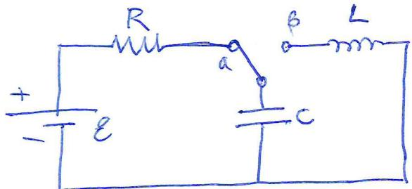
$$E = 12V, \quad R = 10\Omega, \quad L = 0.1H, \quad C = 1\mu F.$$
